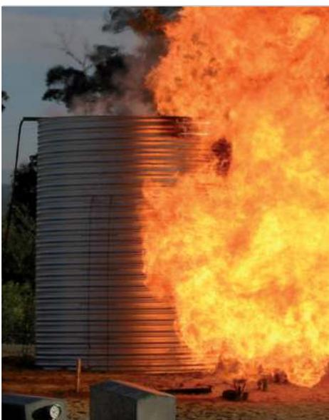
LEFT: WATERPOINT® CLASSIC DURING TESTING AND ABOVE RIGHT: STEEL CONSTRUCTION TANK AFTER FIRE FRONT
